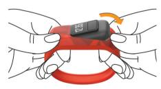
2 Insert the device into the flexible silicone band by stretching the band material around the device.
